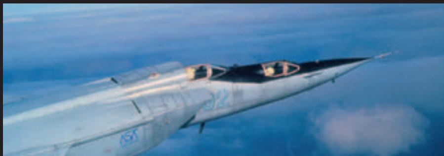
Other than the few other aeroplanes which would have been capable of reaching the height of 27,000 meters, the MiG-25 disposes of essential and special features. In order to reach such a height, a very high maximum speed is required.
