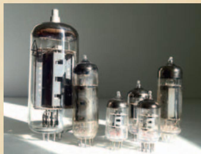
Electronic tubes, the first components of electronics
